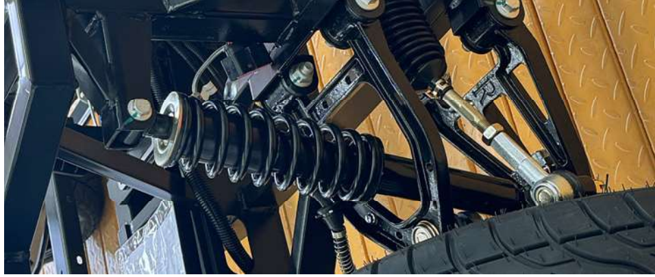
Coilover Suspension With Extra Springs For A Smooth Ride
