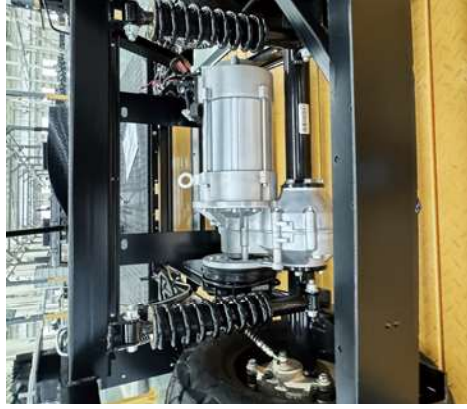
Coilover Suspension With Extra Springs For A Smooth Ride
